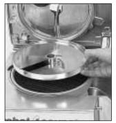
Next, fit the corresponding slicing disc (straightedged blade) and rotate in a clockwise direction to ensure that it is correctly positioned.
