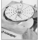
3) If you want to use the lid without the removable partition, screw the cabbage spiral onto the spindle.
