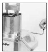
If you have not fitted the cabbage spiral, check that the removable partition has been properly positioned.
